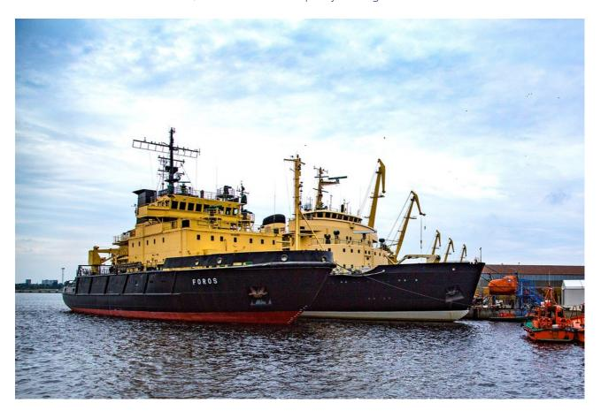
The vessel was purchased for icebreaking operations in the port of Riga. When arriving to Riga, the vessel underwent drydocking in 2015, major renewals were done to steel of hull and auxiliary engines. At its service in Riga the classification society was changed to Maritime Administration of Latvia. FOROS is flying Latvian flag and is maintained in accordance with the requirements of the classification society. Next drydocking is scheduled for December, 2023.
